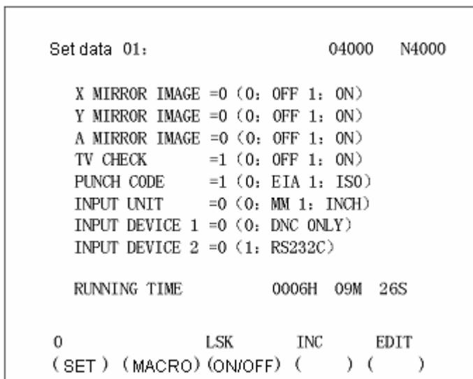
Setting (active when the program protection lock is disabled and inactive when it is locked, which can be switched by parameter)
