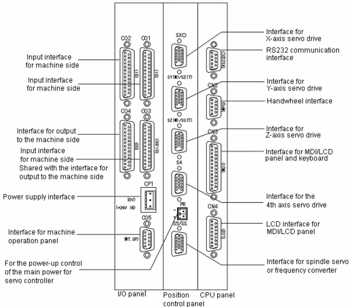
GSK983M system full closed-loop connection diagram
