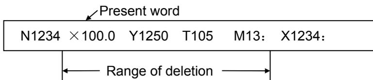
Press the **EOB** and **DELETE** buttons to delete the part before EOB and move the cursor to the underneath of the address character of the next word.
