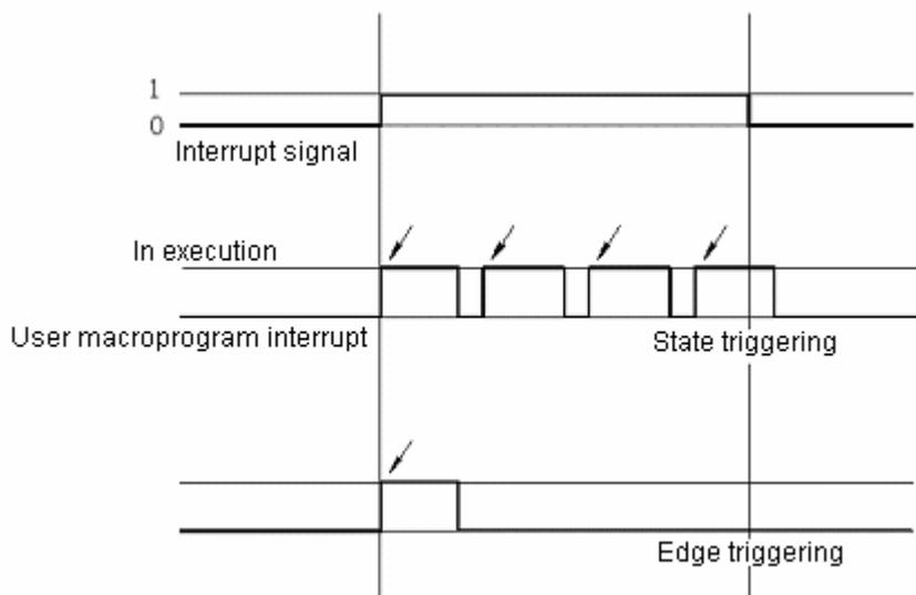
Except special purposes, the actual effects of the two modes are the same (there is not difference in the time from the input of signal to the interrupt of actual execution).
