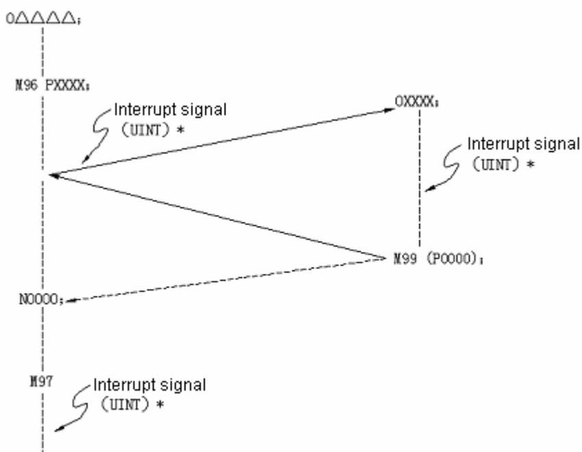
Fig.1: Schematic diagram of user macro program interrupt
