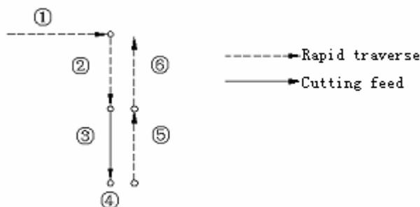
When the result of the fixed circular calculation is not 1, the FEED HOLD indicator illuminates except the block ⑥ of the final cycle. The FEED HOLD indicator illuminates whenever block ① or ② stops.
