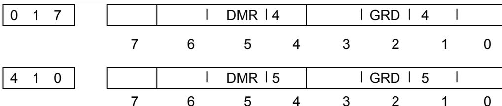
DMRX, DMRY, DMRZ, DMR4 and DMR5 are the measuring override ratio for axes X, Y and Z and the 4<sup>th</sup> axis respectively.
