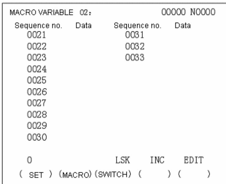
Press the **MACRO** key. Now the local variable and common variable of user macro program are displayed on the LCD screen.
