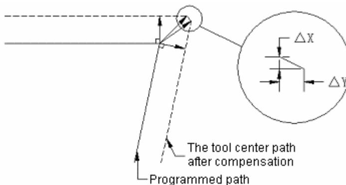
When  $\Delta X < \text{CRCDL}$  and  $\Delta Y < \text{CRCDL}$ , minor stroke is neglected. In this way the influence as a result of workpiece's stop on workpiece may be prevented.
