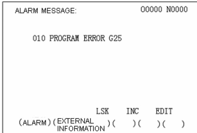
Pressing the **ALARM** soft function key displays the alarm messages as shown in the above figure. Pressing the **OUTMESS** soft function key displays the external information as shown in the above figure.
