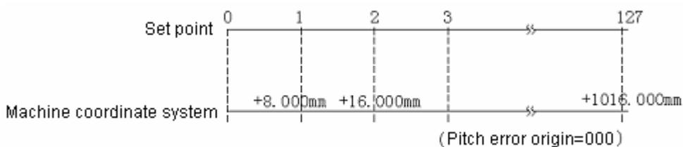
This is the occasion that pitch error compensating clearance (parameters 163 to 166) is 8000.
