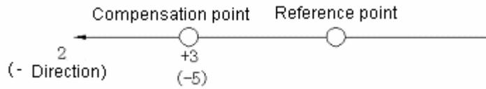
For stroke in positive direction, +3 (-5) shall be compensated by the arrival of the compensation point.
