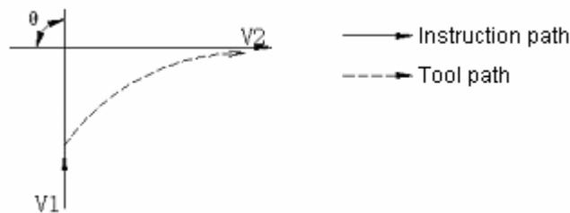
Fig. 4.1 (a): The tool path regarding a turning angle section
