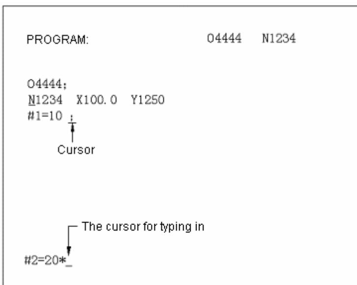
(b) Deletion, insertion and modification of a program
