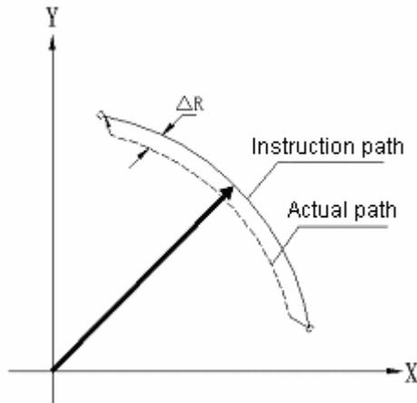
The radius r(mm) and permissible error Δr(mm) of a workpiece are given in actual machining. Permissible speed limit V(mm/sec) can be calculated with the formula (1).
