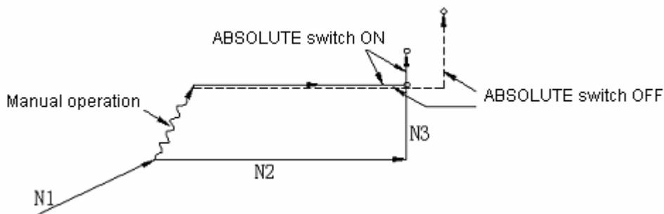
e) When manual operation is followed by an incremental command, then the position that the axis moves to is identical with that is instructed while the MANUAL ABSOLUTE switch is set to OFF.
